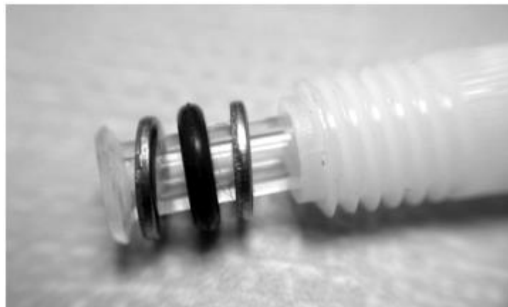
Figure 5.216: Valve flanged end, washers, and o-ring
