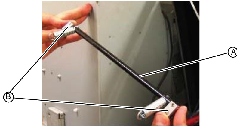
Figure 5.179: Location of spring arm levers on the spring arm rod
