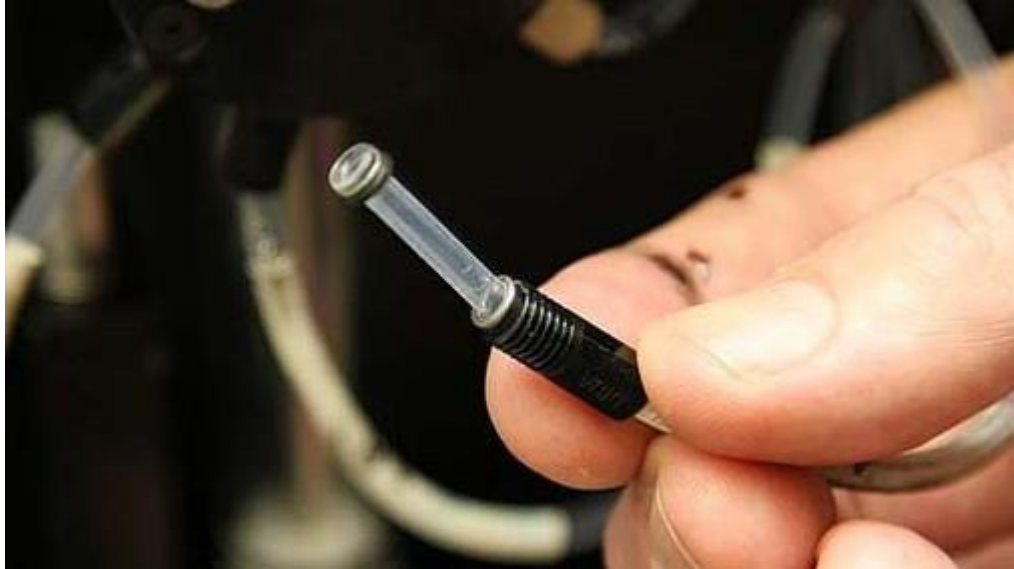
Figure 5.217: Valve fitting pushed back
