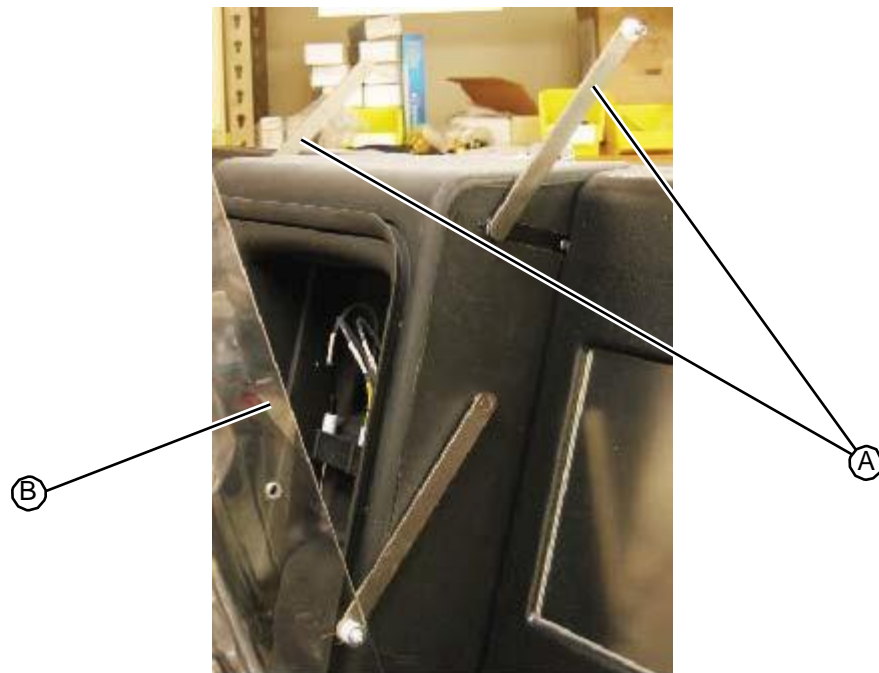
Figure 5.161: Hinge arms rotated up
