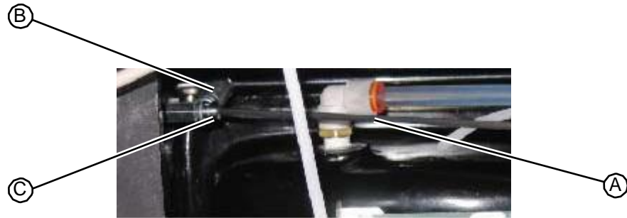
Figure 5.160: Releasing spring fastener
