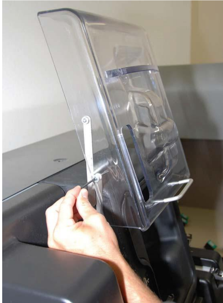
Figure 5.102: Removing vacuum chamber door fasteners with door in open position
