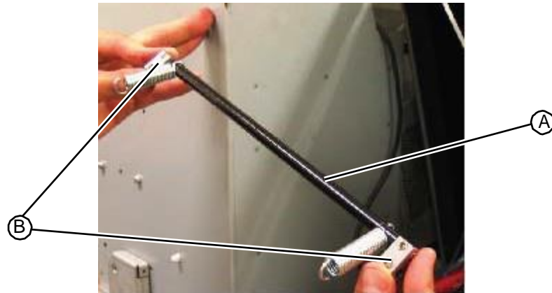
Figure 5.184: Location of spring arm levers on the spring arm rod
