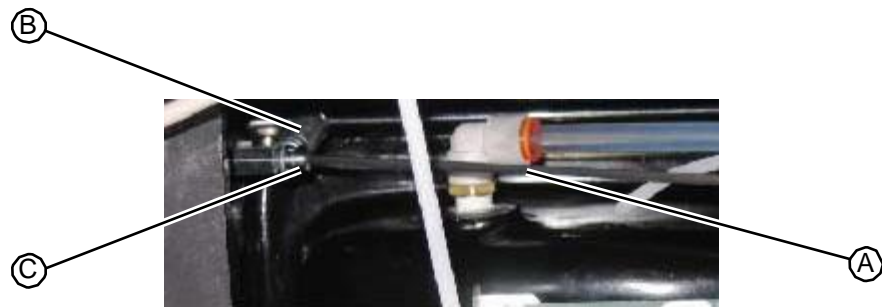
Figure 5.177: Extension spring fastener
