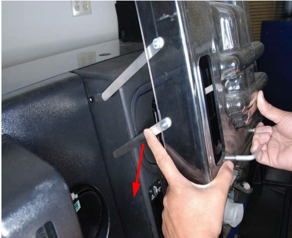
Figure 5.103: Pushing down on the door to rotate it up and forward
