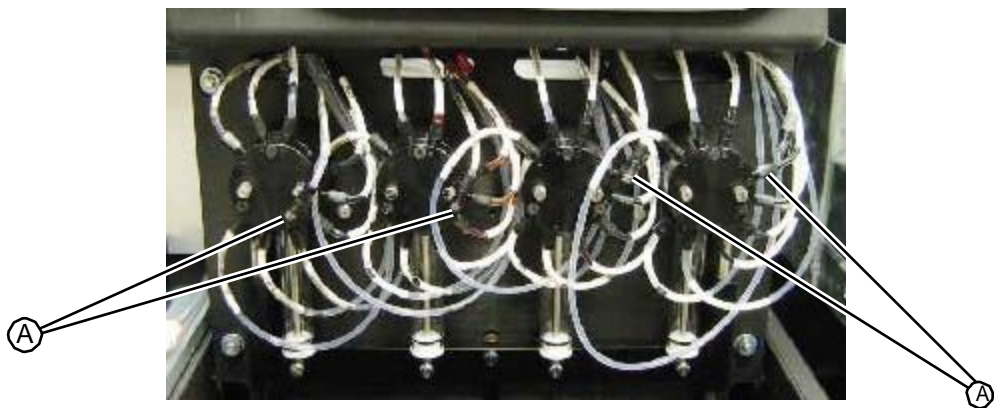
Figure 5.85: Dispense lines disconnected from ink valves
