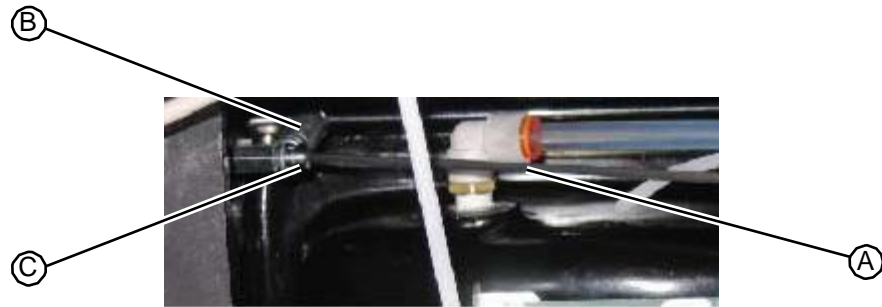
Figure 5.165: Extension spring fastener
