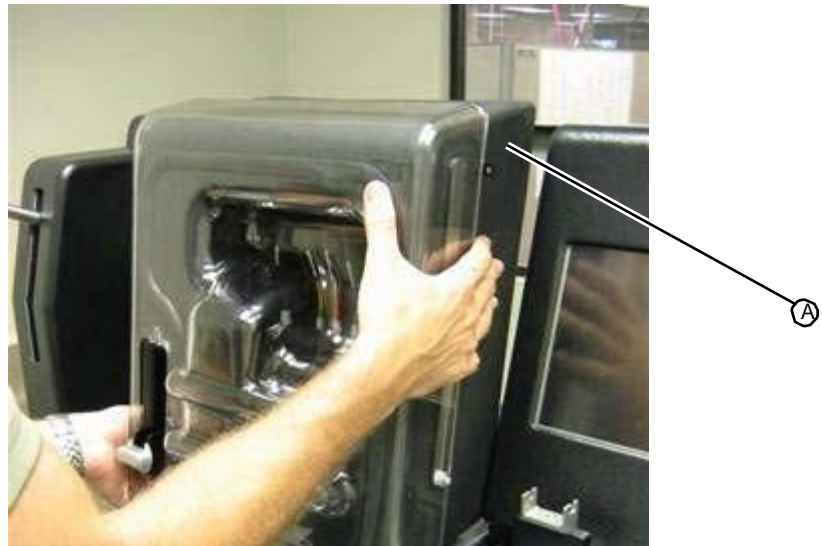
Figure 5.93: Placing the vacuum chamber assembly into the system
