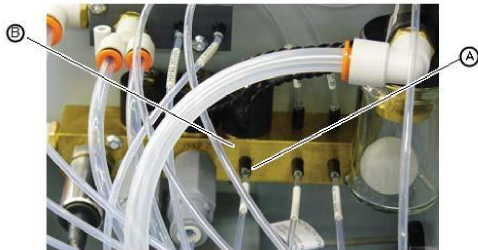
Figure 5.122: HP45 vacuum tubing at waste vacuum manifold
