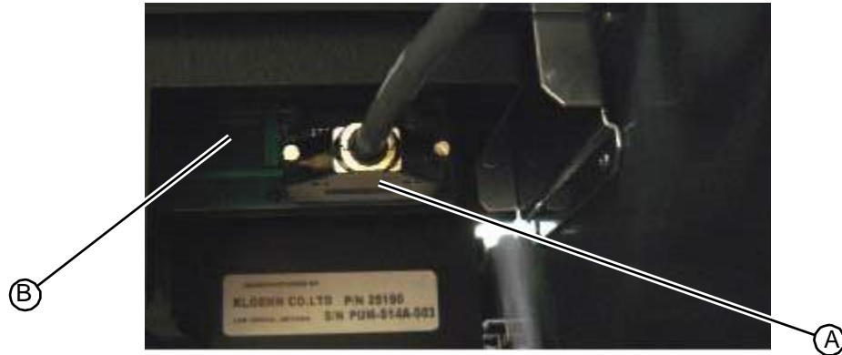
Figure 5.149: DB25 connection on the back of the infusion pump drive system
