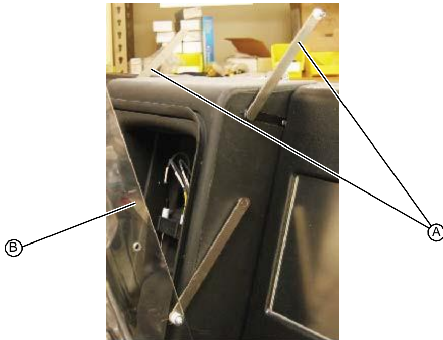
Figure 5.166: Hinge arms rotated up
