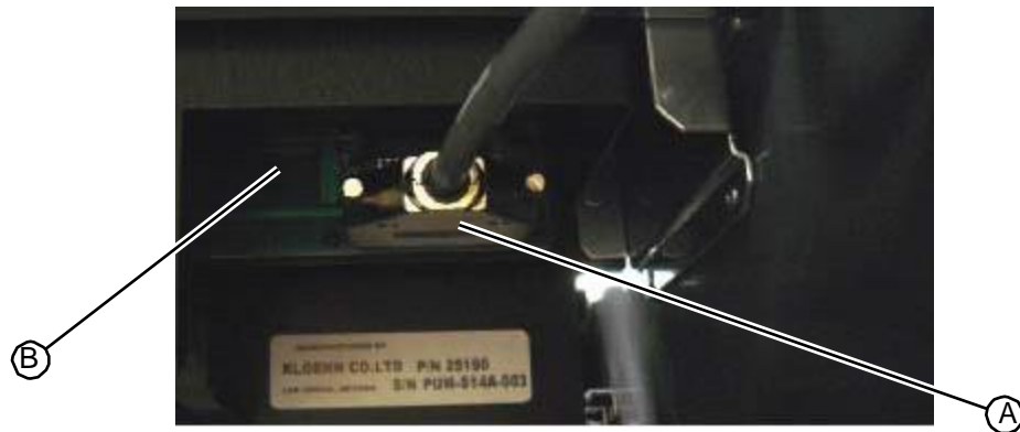
Figure 5.153: DB25 connection on the back of the infusion pump drive system
