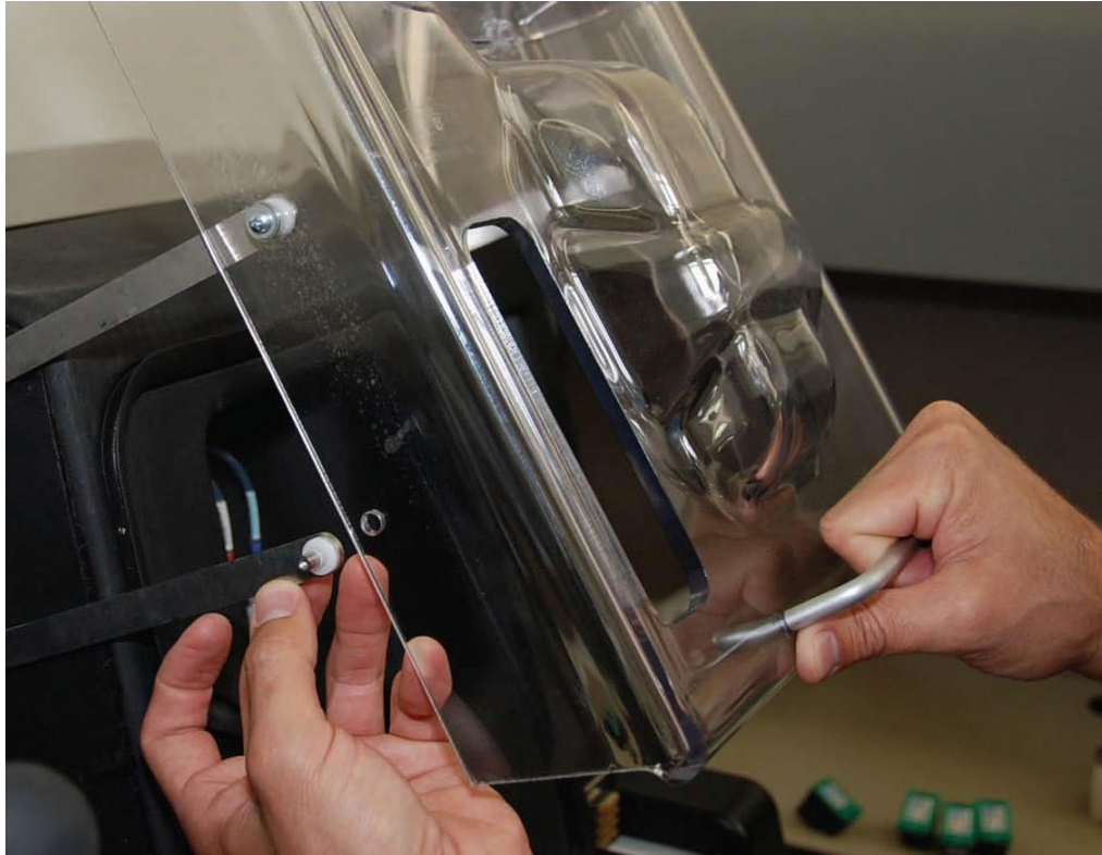
Figure 5.106: Chamber door positioned for re-attachment
