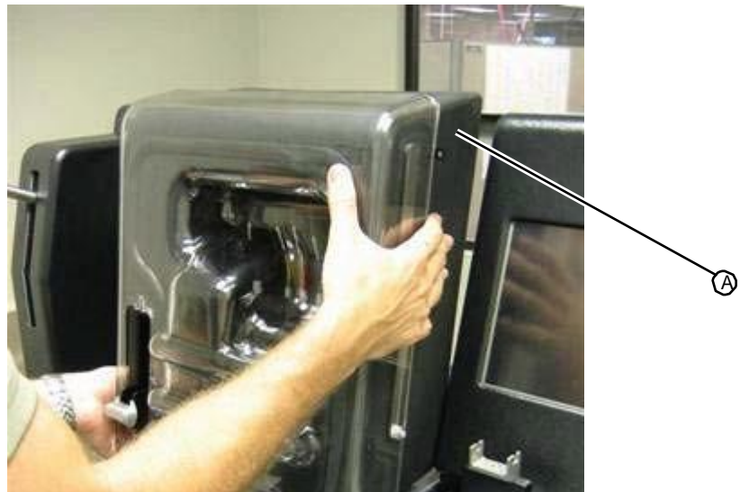
Figure 5.92: Removing the vacuum chamber from the system
