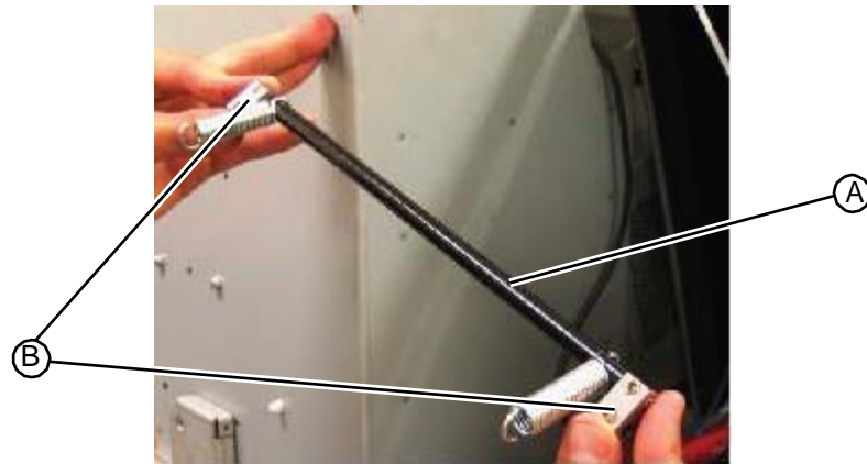
Figure 5.185: Location of spring arm levers on the spring arm rod
