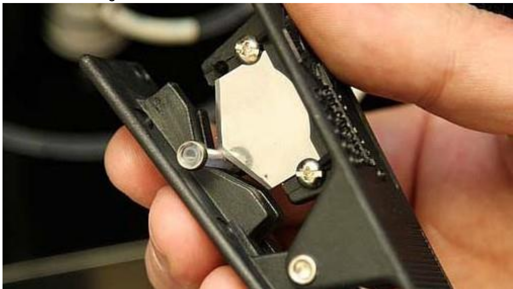
Figure 5.218: Cutting tube with cutter
