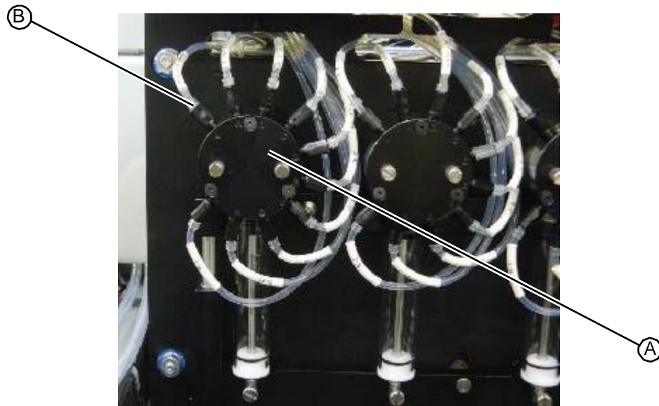
Figure 5.129: HP45 ink line connected to the valve
