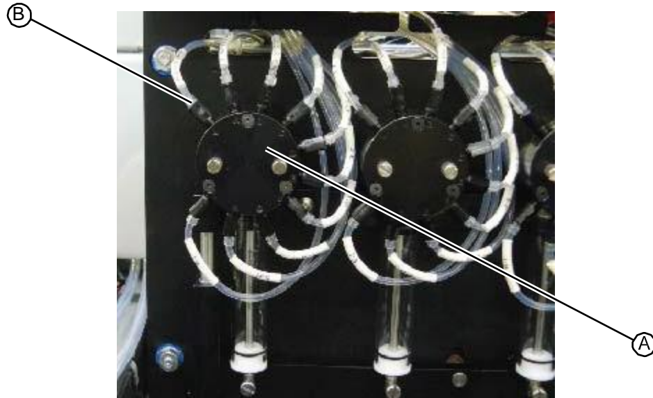
Figure 5.124: HP45 ink line connected to the valve
