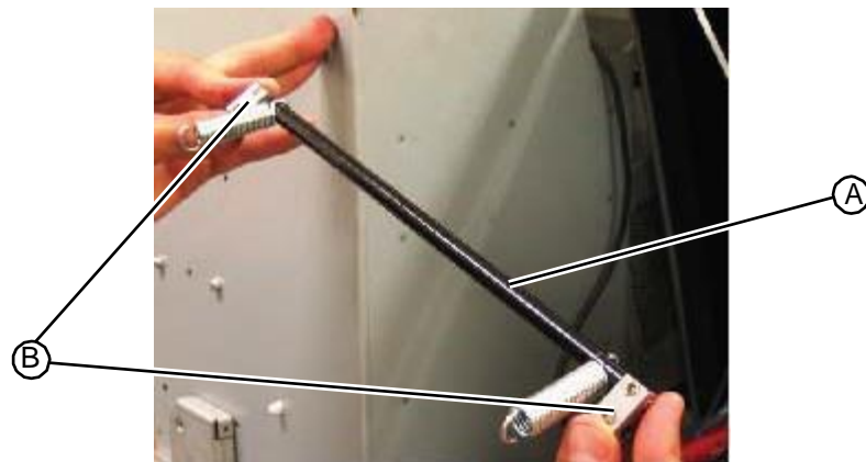
Figure 5.180: Location of spring arm levers on the spring arm rod
